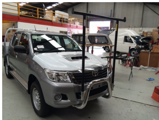
Figure 1: Typical example of a ladder rack fitted to a utility
