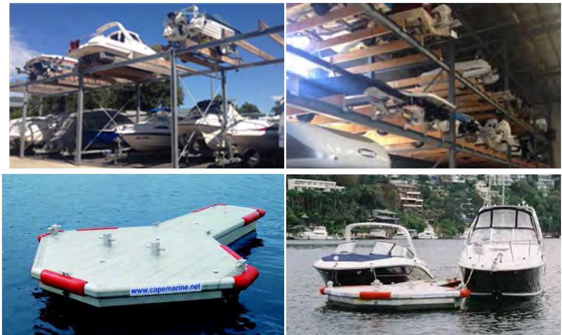
Figure 8 – Dry storage at Kurnell (top) and an alternative mooring apparatus 1 (bottom)
