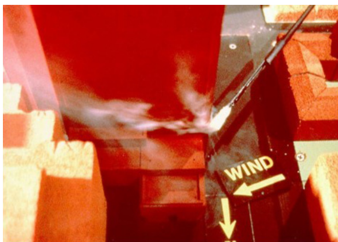
Figure 28: Test Model -Wall vortex and separated flow both apparent at the intersection of a tall building and low-rise podium. This vertical vortex has the potential to yield the largest magnitude negative cladding design pressure on a project (after ASCE Webinars 2005-2012)
