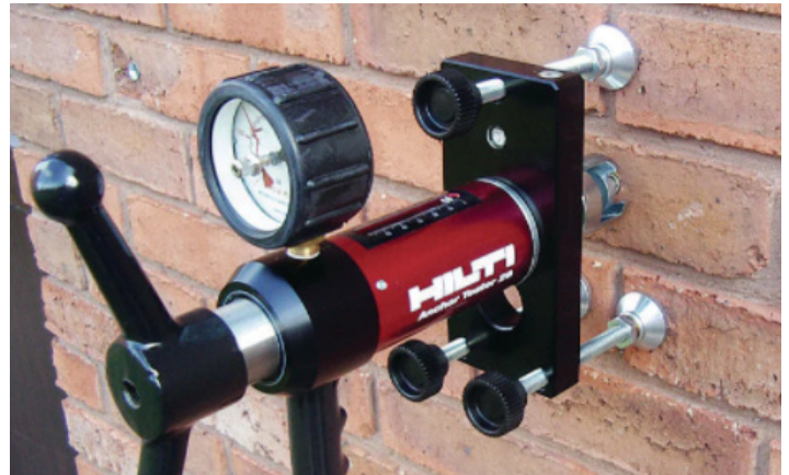
Figure 8: Masonry pull-out test
