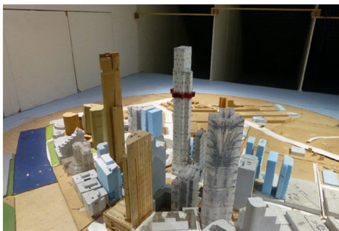
Figure 27: Wind Tunnel Testing – Turntable of modelled cityscape with upwind spires and roughness behind the photographer
