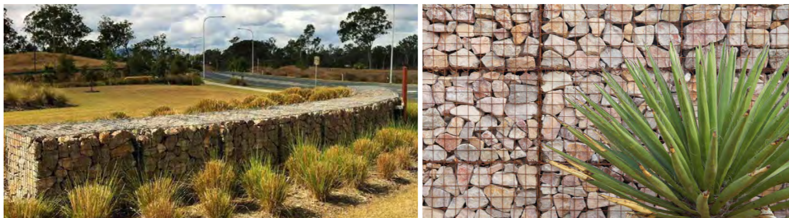
Figure 53. Precedent images of gabion feature walls
