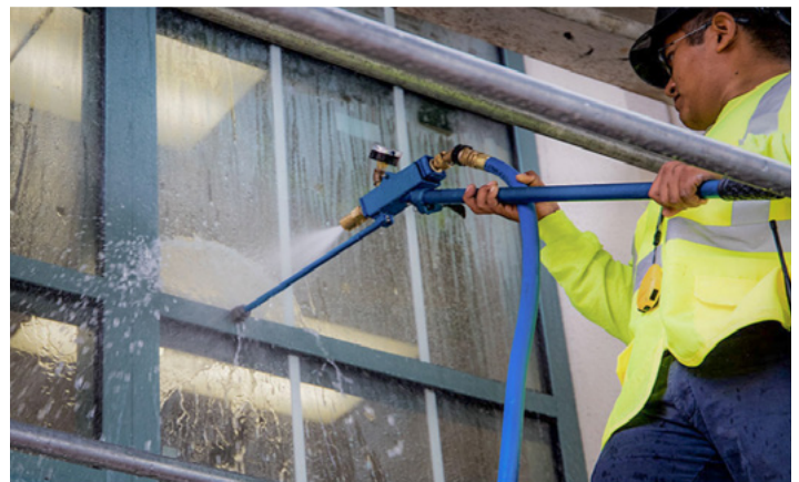
Figure 5.7: Window hose testing
