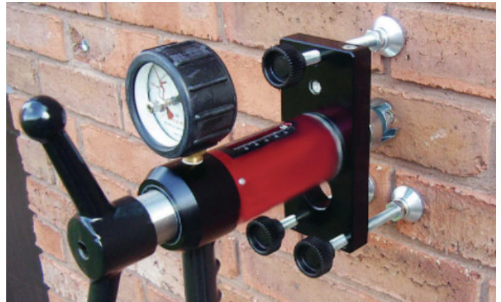
Figure 5.6: Masonry pull-out test
