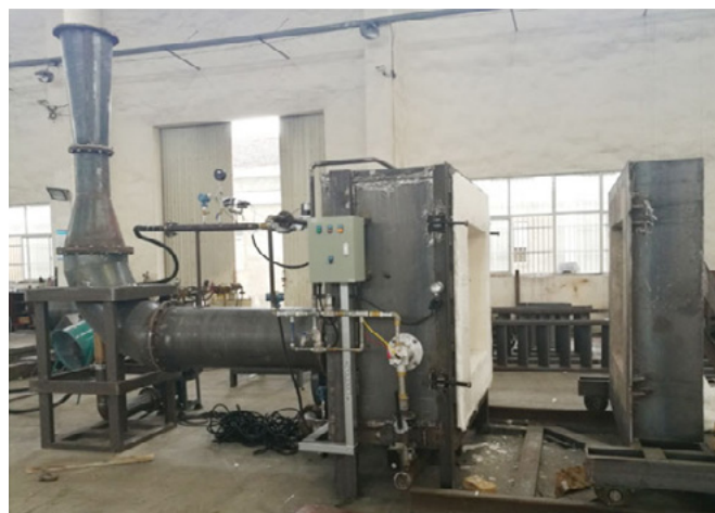
Figure 10.3: AS 1530.4 Testing Rig
