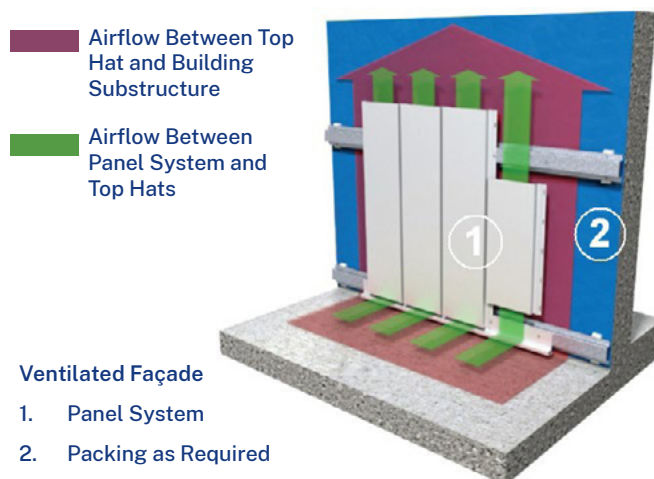
Figure 16.2: Ventilated façade principles (airflow)
