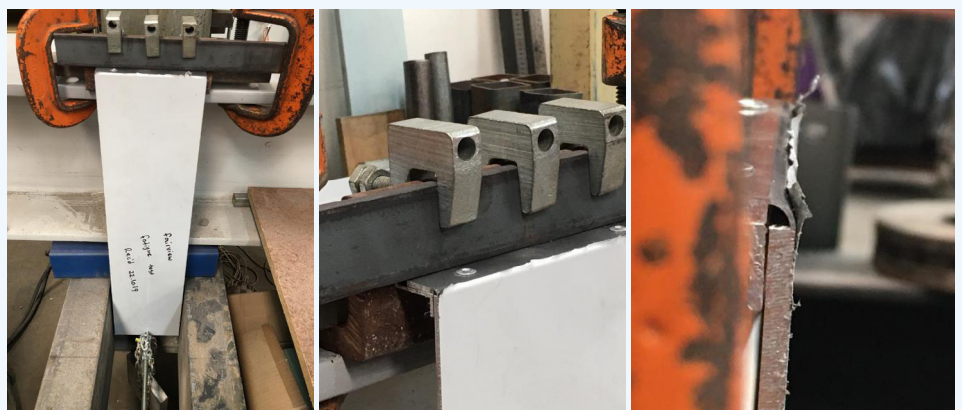
Figure 16.8: Fatigue testing of solid aluminium panels
