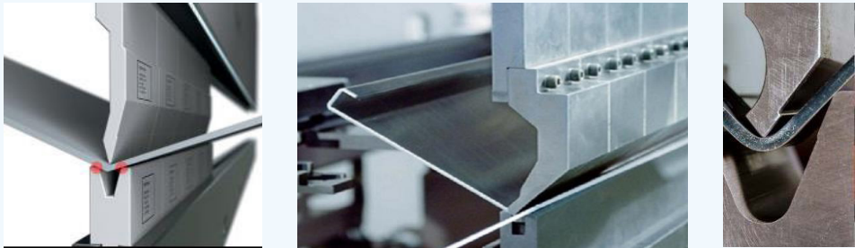
Figure 16.4: Folding of aluminium sheet using mechanical methods including break pressing
