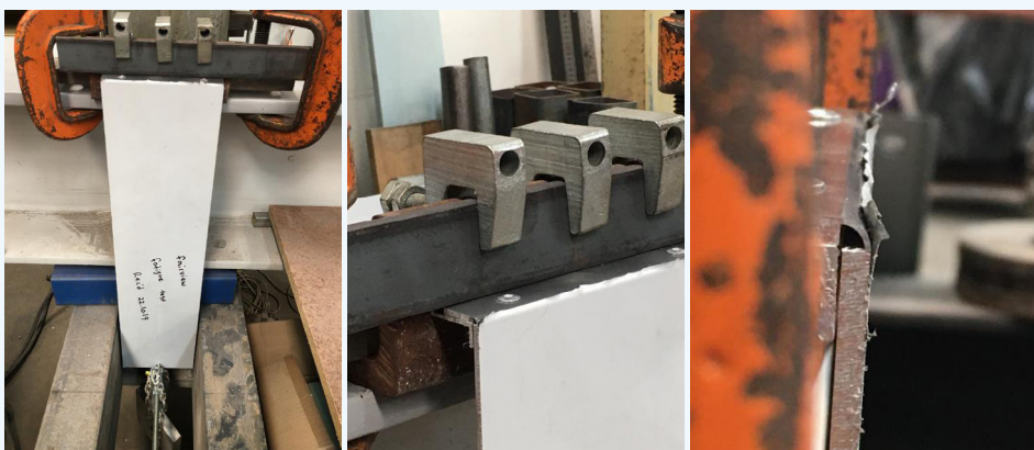
Figure 16.8: Fatigue testing of solid aluminium panels
