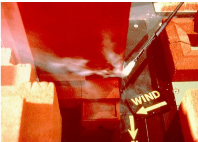
Figure 14.4: Test Model -Wall vortex and separated flow both apparent at the intersection of a tall building and low-rise podium. This vertical vortex has the potential to yield the largest magnitude negative cladding design pressure on a project (after ASCE Webinars 2005-2012)
