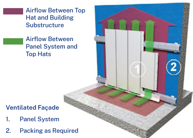
Figure 16.2: Ventilated façade principles (airflow)
