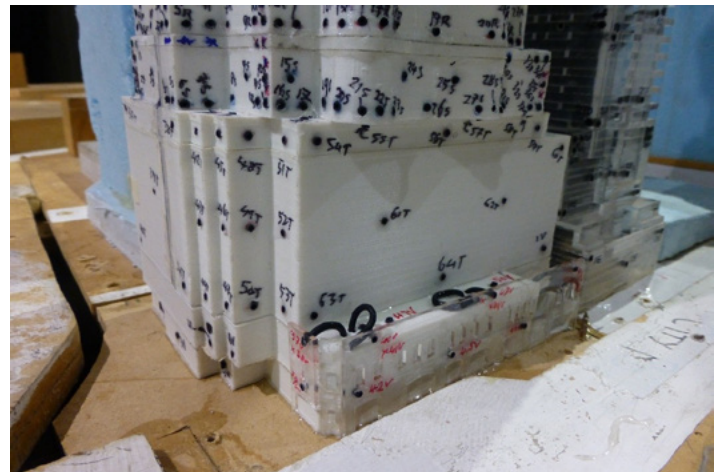
Figure 14.6: Wind Tunnel Testing - Pressure taps at varying building geometry
