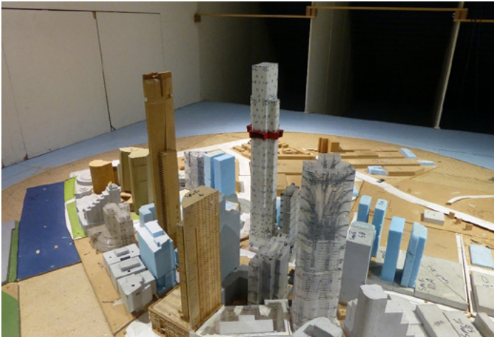
Figure 14.3: Wind Tunnel Testing – Turntable of modelled cityscape with upwind spires and roughness behind the photographer
