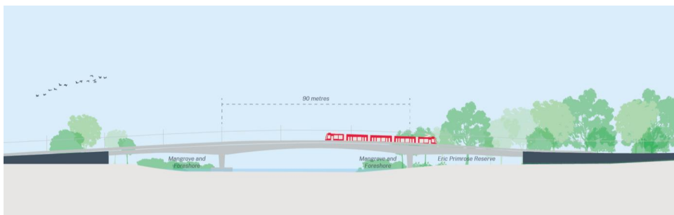
Figure 6.15 Indicative elevation of bridge between Camellia and Rydalmere (viewed from the east)
