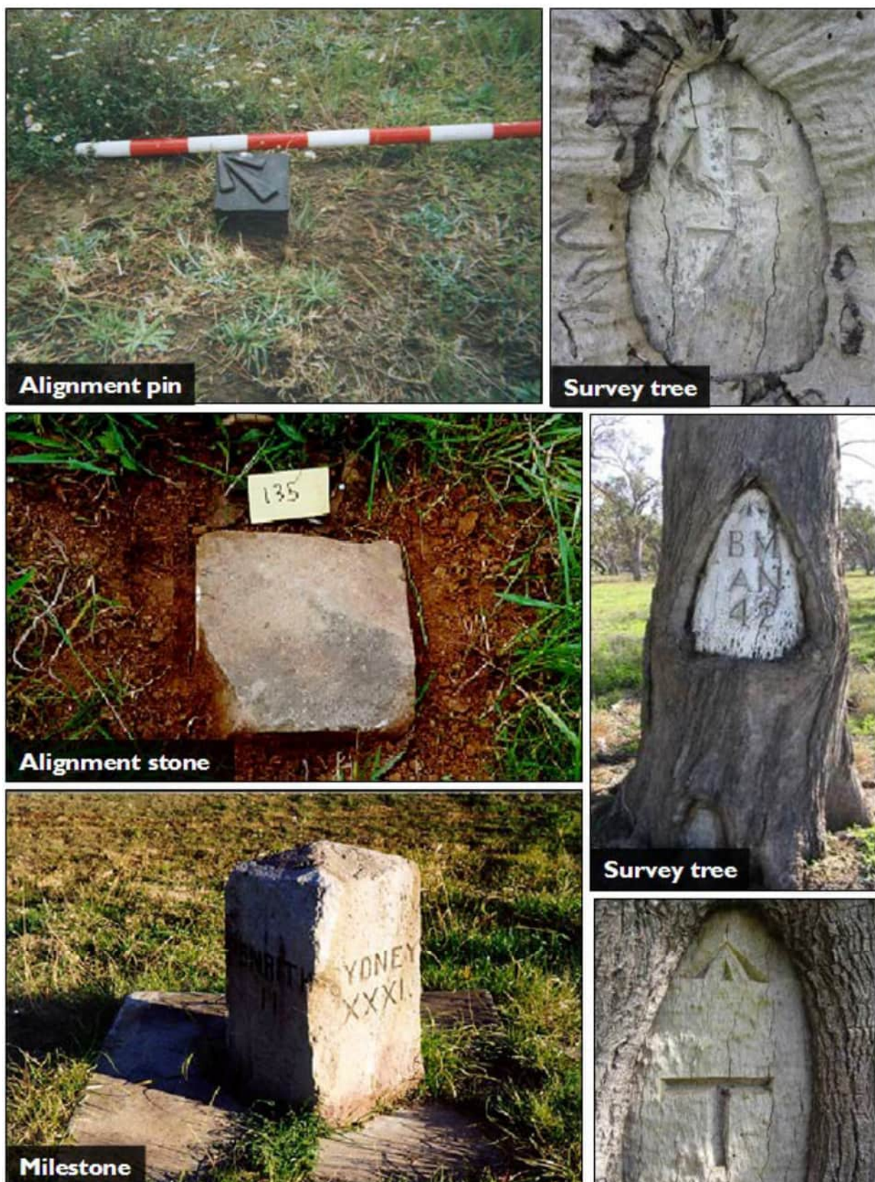
Figures: Top left-hand corner continuing clockwise: alignment pin (Great Western Highway, Wentworth Falls); survey tree (MR7, Albury); survey tree (Kidman Way, Darlington Point, Murrumbidgee); survey tree (Cobb Highway, Deniliquin); milestone (Great Western Highway, Kingswood, Penrith); alignment stone (near Guntawong Road, Riverstone). Please note survey marks may have additional statutory protection under the Surveying and Spatial Information Act 2002 .
