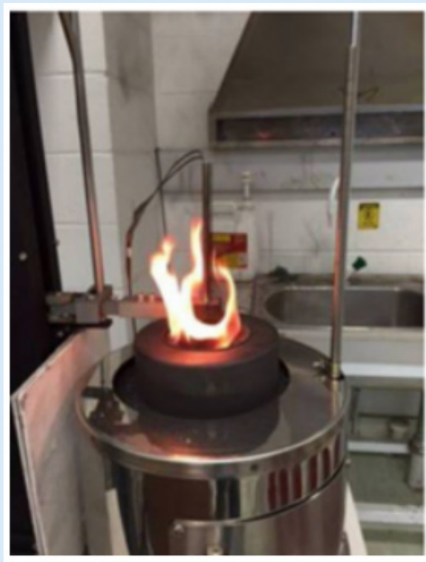
Figure 5: Fire test to AS 1530.1 (Source: ISpecify)
