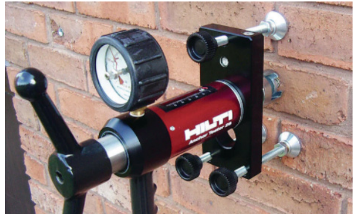
Figure 8: Masonry pull-out test
