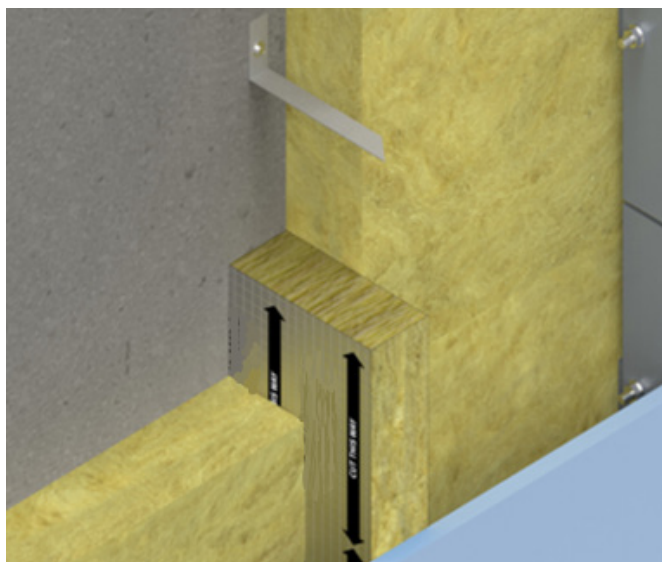
Figure 15: Closed-state cavity barrier
