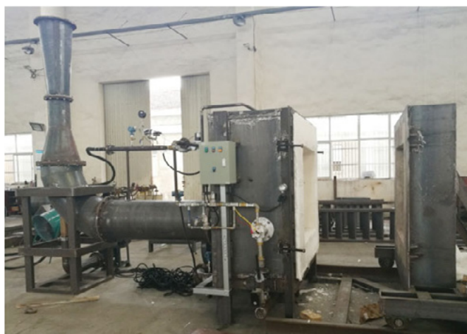
Figure 16: AS 1530.4 Testing Rig
