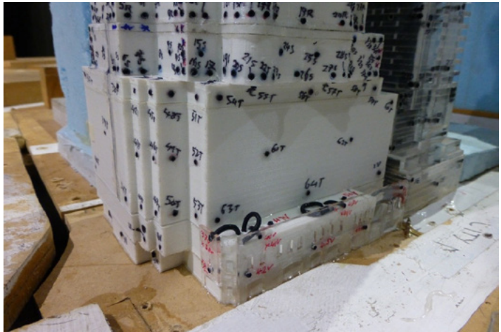
Figure 30: Wind Tunnel Testing - Pressure taps at varying building geometry
