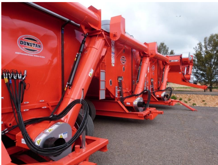
Figure 19: Chaser bins, used to transport agriculture produce to a road train or other hauling device, at Dunstan Farmers Engineering. Photo credit: Campaspe Shire Council.
