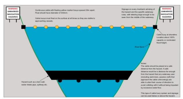
Image: The above diagram provides an example of continuous cable with floating yellow marker buoys, spaced 25 meters apart. Float should have a minimum diameter of 300mm. The cable of aqua buoys should float on the surface at all times, so they are visible to approaching vessels.
