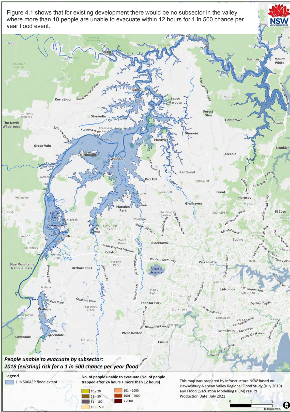
Figure 4.1: People unable to evacuate by subsector: 2018 (existing) risk for a 1 in 500 chance per year flood
