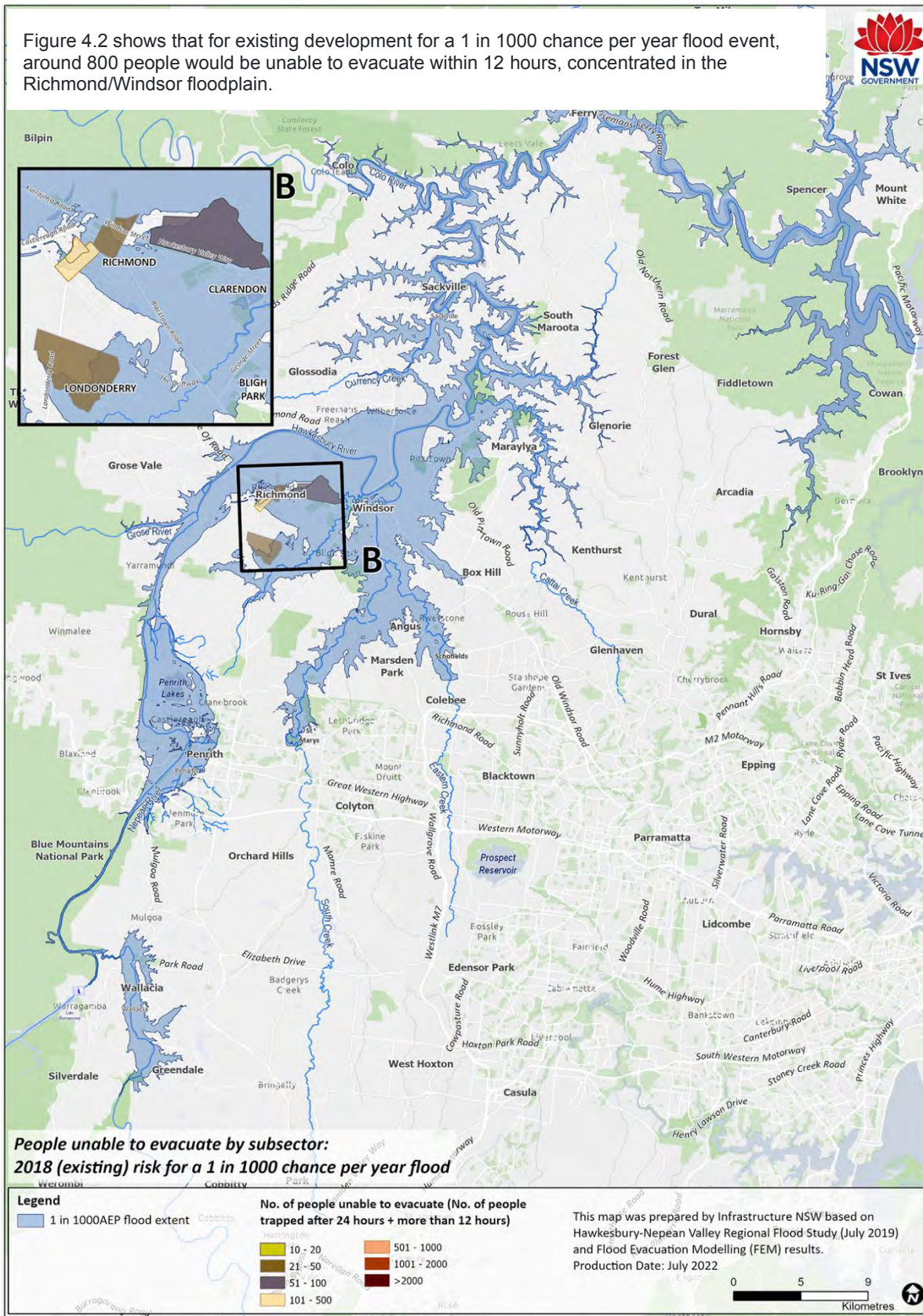
Figure 4.2: People unable to evacuate by subsector: 2018 (existing) risk for a 1 in 1000 chance per year flood
